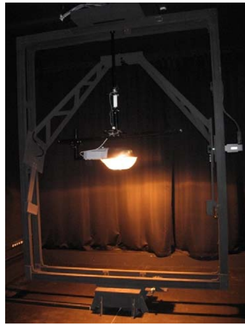
Figure 2. Near-field goniophotometer during measurement of street lighting luminaire with high pressure sodium lamp
