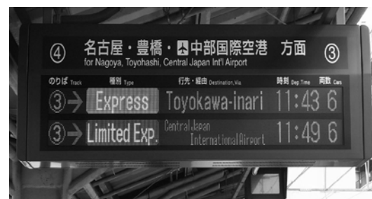
Figure 1 LED-type information display board within the station
