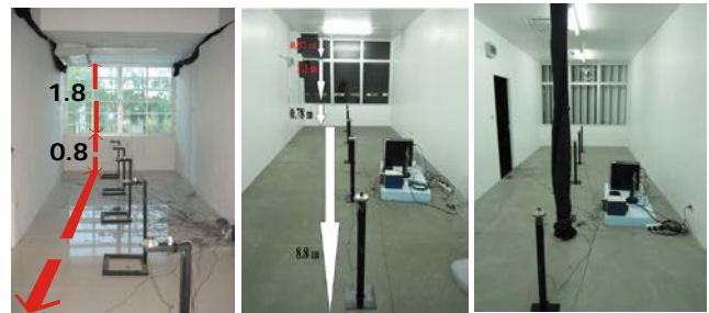
Figure 2 The experimental rooms with illuminance sensors.
